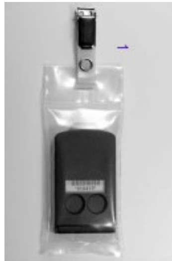
Albedo- (Thermoluminescence) Dosimeter: n ( \beta ) \gamma x-ray Neutrons > 0.5 \text{ eV}
